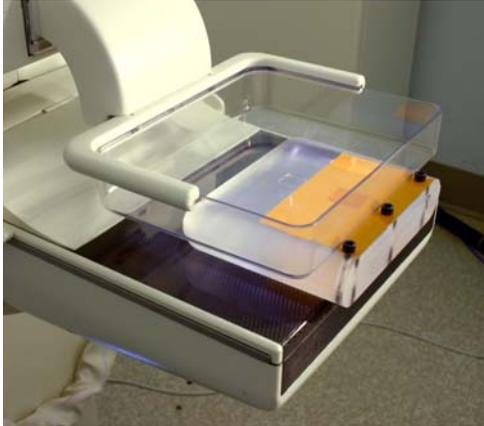
**Figure 2:** ACR FFDM Accreditation Phantom positioned for imaging
