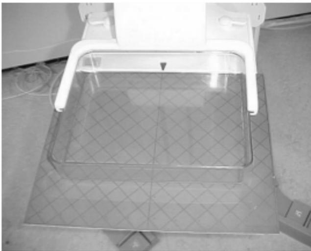
Figure 9: Geometric Distortion Test Tool
