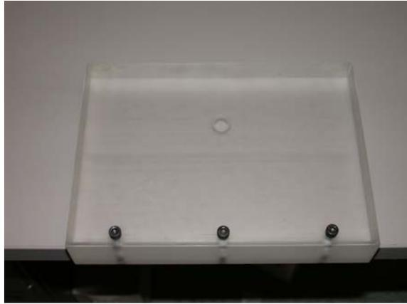
**Figure 4:** Image of a uniform phantom suitable for artifact evaluation and MGD estimation.
