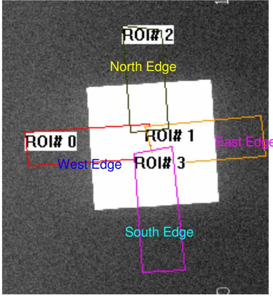
Illustration of the effect of sampling size along the edge of an MTF tool. Notice the color legend on left and right are different. On the right, ROI#1 is cropping the "East Edge", ROI#0 for "West Edge", ROI#2 for "North Edge" and ROI#3 for "South Edge", like you are reading a map normally. It is obvious that the longer the sample along the edge, the smoother the resultant MTF graphs.
